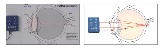
**Near sighted eye**: Place the eye lens no 2 directly the behind the line O2 and correction lens no 5 between the line O1 and O2. Display rays parallel to the optical axis intersect after passing through uncorrected eye lens at one point of the optical axis before the retina.
